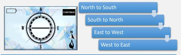
To determine the depth of the discovered target, stand above target and turn 45 degrees
